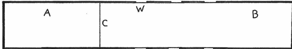
Fig. 2a. Schematic Diagram of Shock Tube. A, high pressure section; B, low pressure section; C, diaphragm; W, quartz windows.
