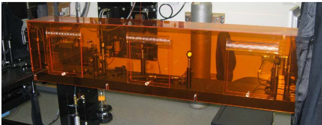
Figure 4-2: Photograph of “the bridge” with orange acrylic optical guard installed. The bridge contains the laser pulse measurement photodiode, as well as apertures and sheet-forming optics. Beam path is from right to left.
