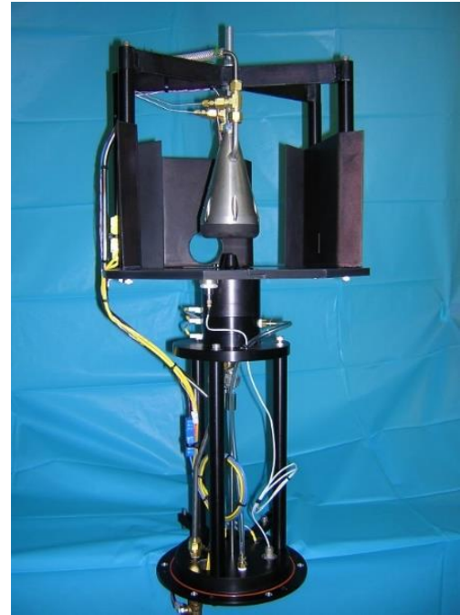
Figure 2-3: Flat-flame burner assembly. (Left) Simplified three-view showing the nozzle, stagnation body and stagnation body support structure. (Right) Photo of burner assembly along with chamber base-plug and interconnecting support rods. Stagnation body height, H , is shown as 21 mm. This corresponds to an H/D = 1.5 , which is the value used for all experiments.
