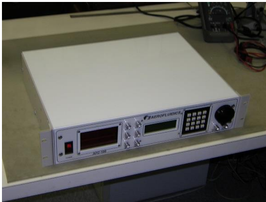
Figure 2-7: The AFC-100 acoustic forcing controller. The instrument was custom engineered and built to solve many of the difficulties previously discovered in the experimental technique. Details of its design and resulting features can be found in appendix F.
