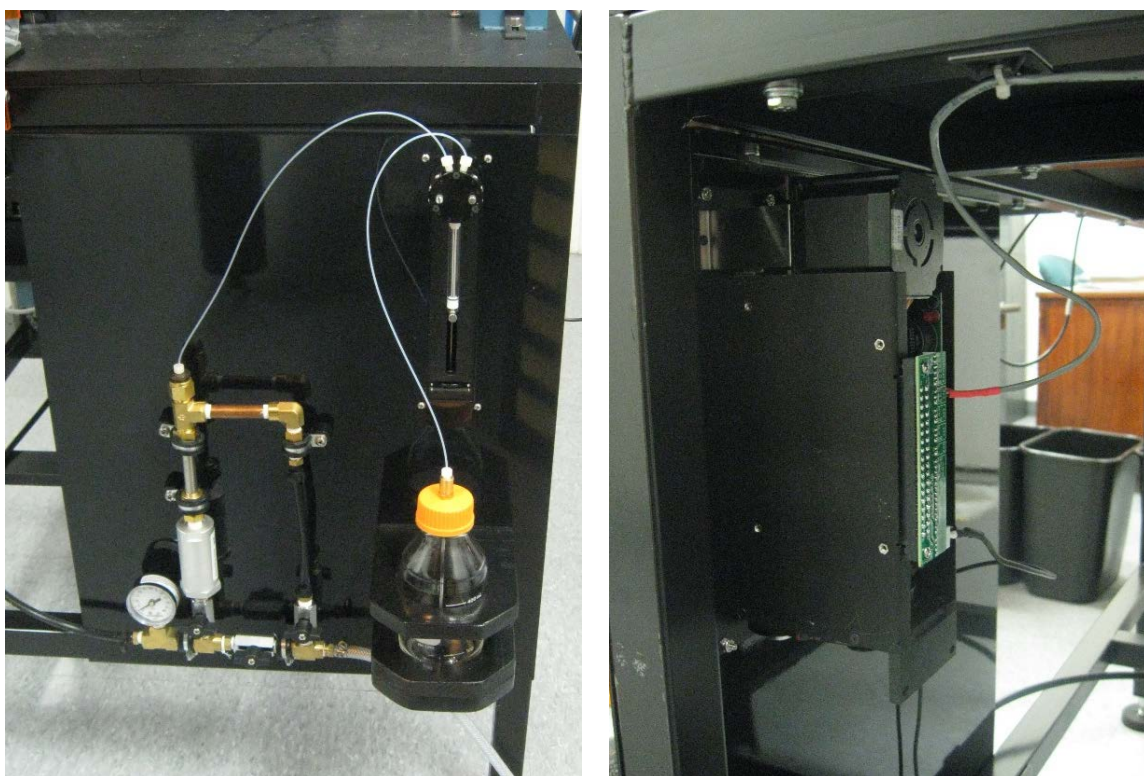
Figure C-1: Left – acetone seeding panel installed on the side of the experiment table. A glass Pyrex bottle serves as the acetone reservoir. The clear, braided PVC hose in the lower right brings the incoming fuel/air mixture to the panel. The black polypropylene hose in the lower left carries the seeded mixture to the burner. Right – view of the back side of the panel showing the body of the precision syringe pump.
