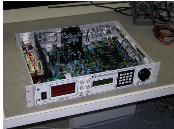
Figure 2-7: The AFC-100 acoustic forcing controller. The instrument was custom engineered and built to solve many of the difficulties previously discovered in the experimental technique. Details of its design and resulting features can be found in appendix F.
