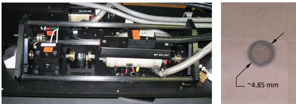
Figure E-5: Left – redesigned Nd:YAG laser oscillator cavity. Right – oscillator output burn (near-field) taken with Kodak Linagraph paper, type 1895.
