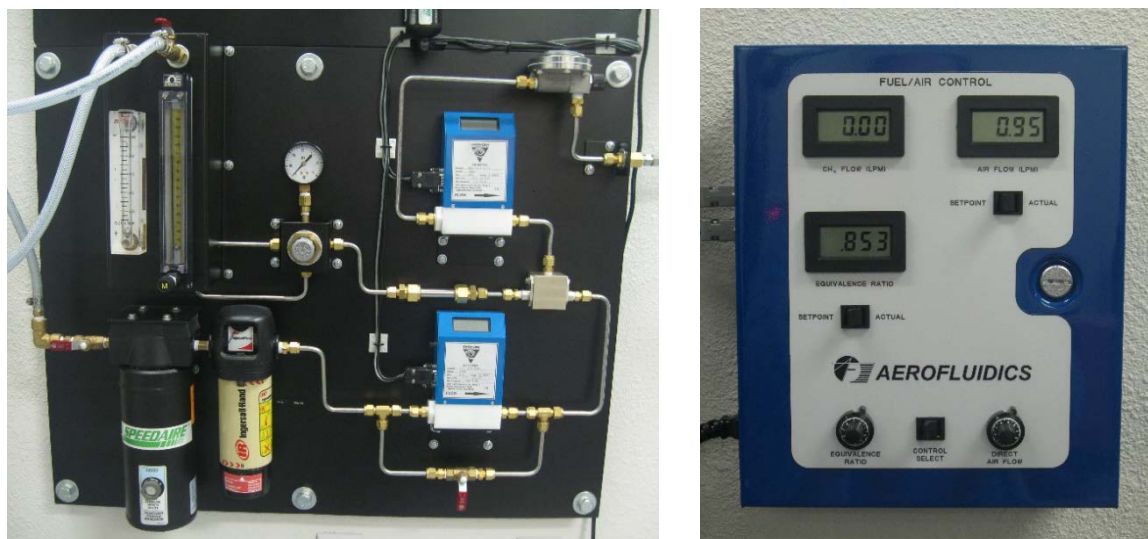
Figure B-9: Left – mixing panel used to generate fuel/air mixture for experimental burner. Right – mixing system control electronics.
