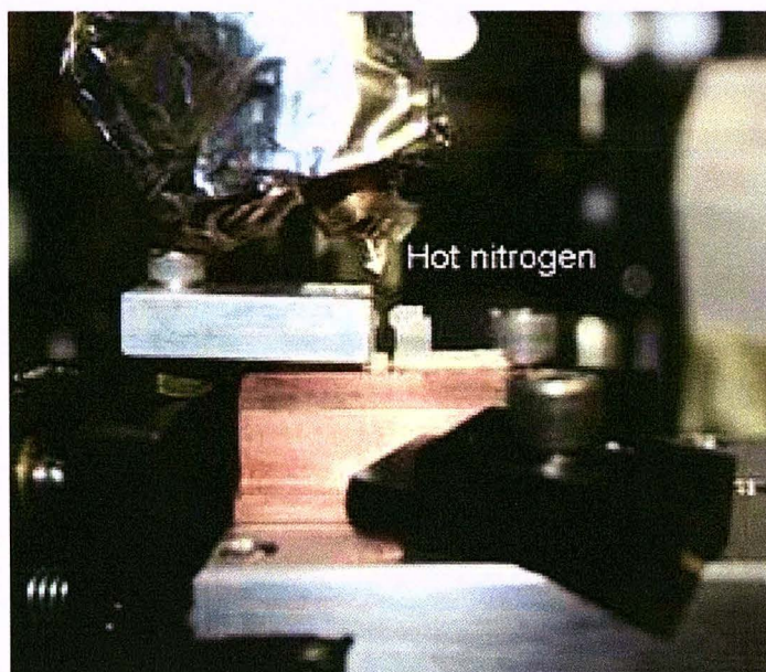
Figure 3.7: We heated our cavity with hot nitrogen in order for the H27DUHV epoxy to cure. Depending on the distance from the tip of the copper tube and the angle, the temperature near the tip ranged from approximately 150 °C to 200 °C.
