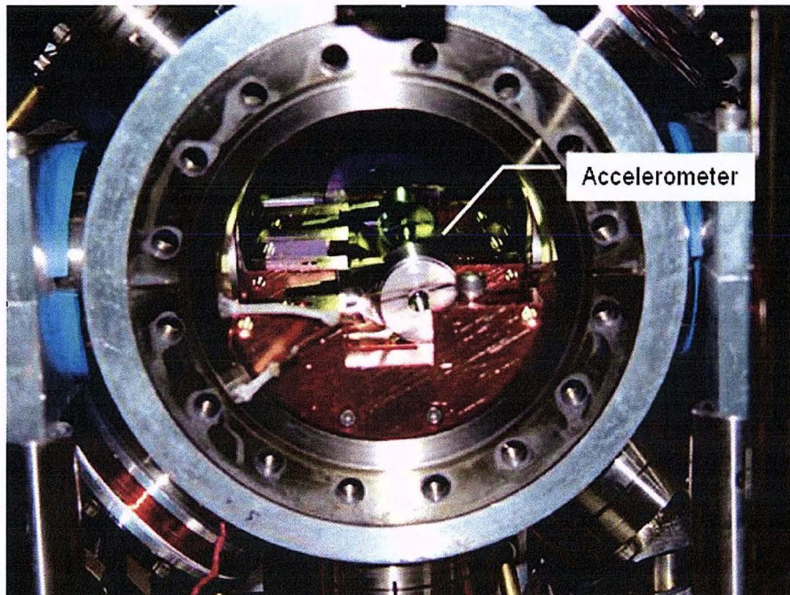
Figure 3.2: The accelerometer on the top stage of the VIS, inside the vacuum chamber.
