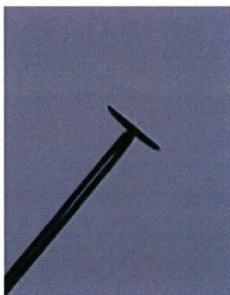
Figure 7: Anoth photo taken of a plate grown in DC2. This time the view is from the side and shows the same profile as the one generated by the SDAK computer simulation.
