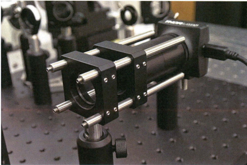
Fig. 2-10: CCD camera used in the set up. We installed two lens tubes to block background light.
