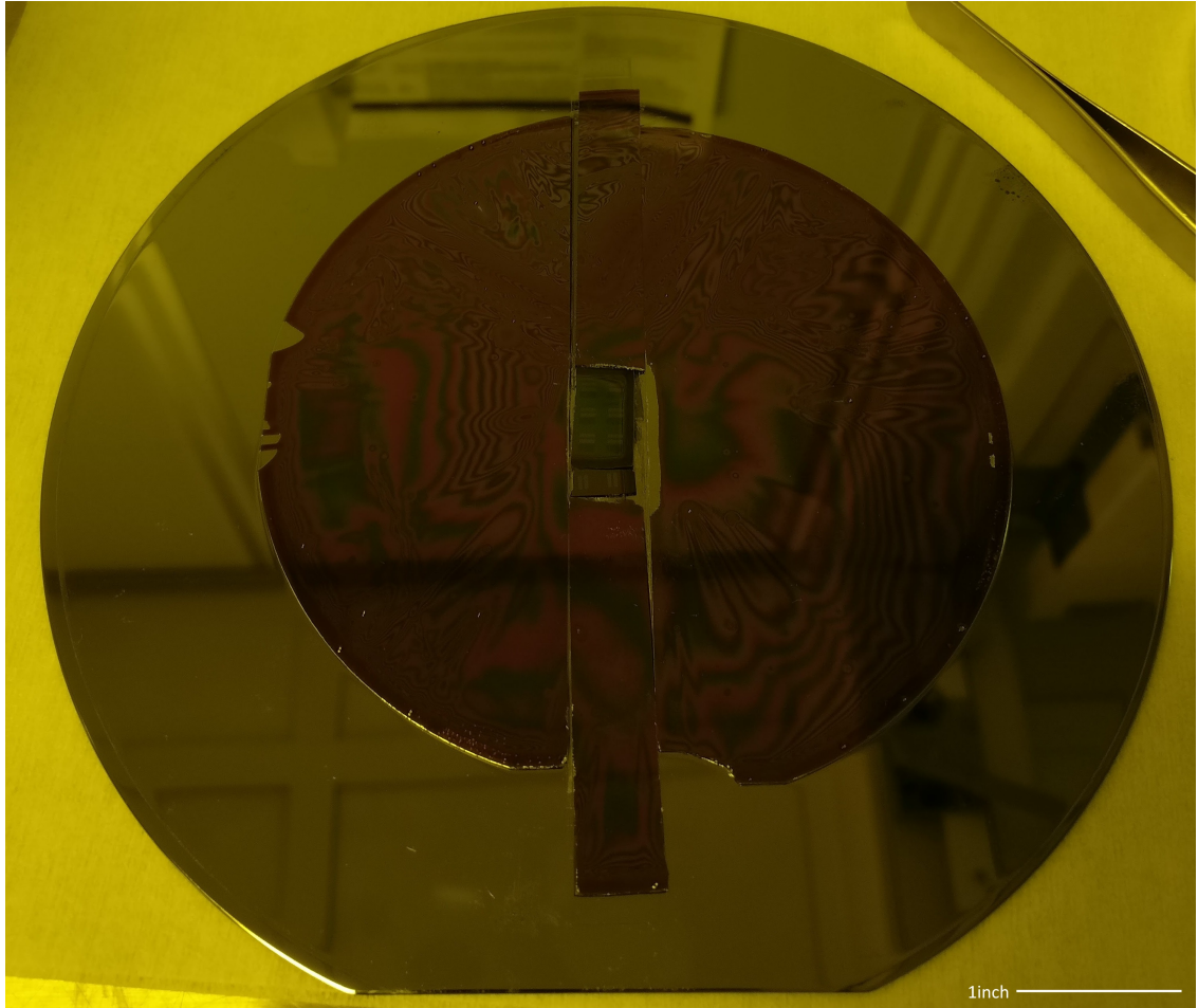
Figure A.11: Carrier wafer with photoresist coated wafer in addition to test samples in center. This technique is used to simulate the properties of the etch when applied to a wafer-scale process as opposed to chips alone.
