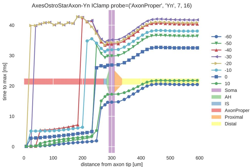
Figure 3.15: The time required for the axon tip to reach maximum membrane voltage (y-axis in  $\mu$ s) when a 0.1 ms square current pulse is injected at that distance from the axon tip (x-axis) with the current necessary (see Fig. 3.6) to reach the specified membrane voltage (see legend).
