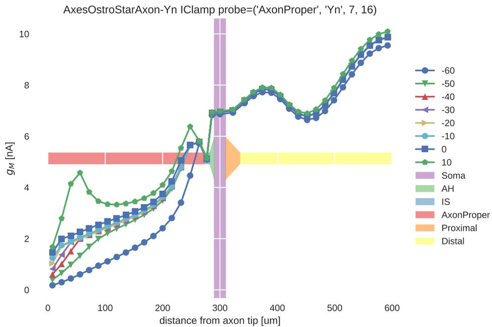
Figure 3.14: Current amplitude (y-axis in nA) necessary for a single square current pulse 0.1 ms long injected at that distance (x-axis in  $\mu\text{m}$ ) from the axon tip to cause the specified membrane voltage (see legend:  $-60$  mV to  $10$  mV in steps of  $10$  mV) at the axon tip.
