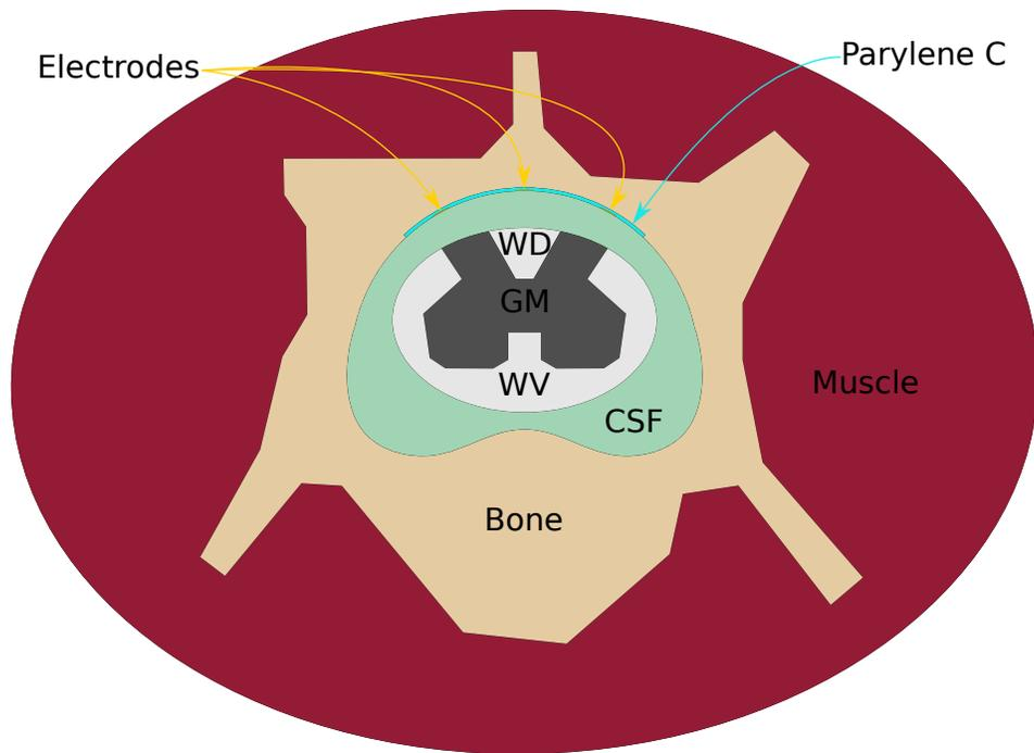
Figure 2.6: After the sketch in Fig. 2.5 was extruded to a length of 23.1 mm, 10  $\mu\text{m}$ -thick electrodes were placed in the parylene. This figure shows a slice through one of the electrode rows. The cerebrospinal fluid is labeled CSF. The dorsal white matter, ventral white matter, and gray matter are labeled WD, WV, and GM respectively. See Fig. 2.7 for a close up view of the electrodes.
