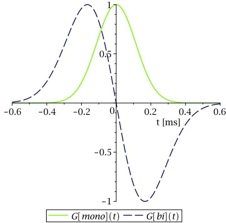
Figure 2.11: Plots of a Gaussian monophasic pulse  $G_{mono}(t, \varsigma_{mono})$  and Gaussian biphasic pulse  $G_{bi}(t, \varsigma_{bi})$ . Where  $\varsigma_{mono} \approx 112.84 \mu\text{s}$  and  $\varsigma_{bi} \approx 166.04 \mu\text{s}$  cause  $G_{mono}(t, \varsigma_{mono})$  and  $G_{bi}(t, \varsigma_{bi})$  to have the same amount of power as a square pulse with width  $w = 200 \mu\text{s}$  and a biphasic square pulse with width  $2w$  respectively.
