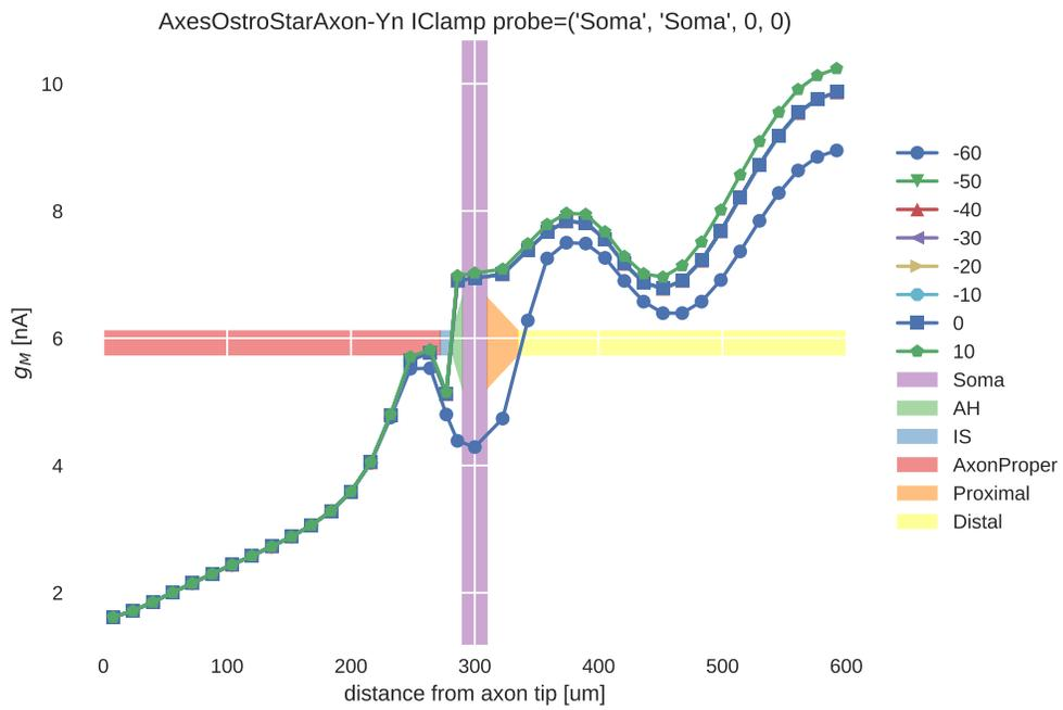
Figure 3.16: Current amplitude (y-axis in nA) necessary for a single square current pulse 0.1 ms long injected at that distance (x-axis in  $\mu\text{m}$ ) from the axon tip to cause the specified membrane voltage (see legend:  $-60$  mV to  $10$  mV in steps of  $10$  mV) at the soma.
