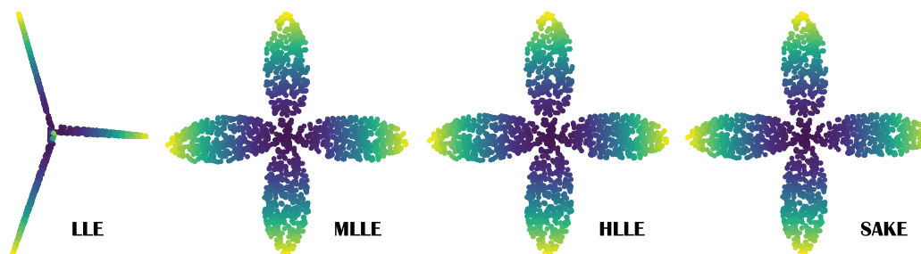
Figure B.2: Local Methods for Noiseless Petals. From a 3D sampling of 4-petal shaped portion of a sphere (see Fig. 4.1), local methods such as Modified LLE [203], Hessian LLE [71], or SAKE have no issue with the non-convexity of the intrinsic geometry (unlike Isomap), and give results nearly equivalent to PTU. A notable exception is LLE [155], which returns a near degenerate solution.
