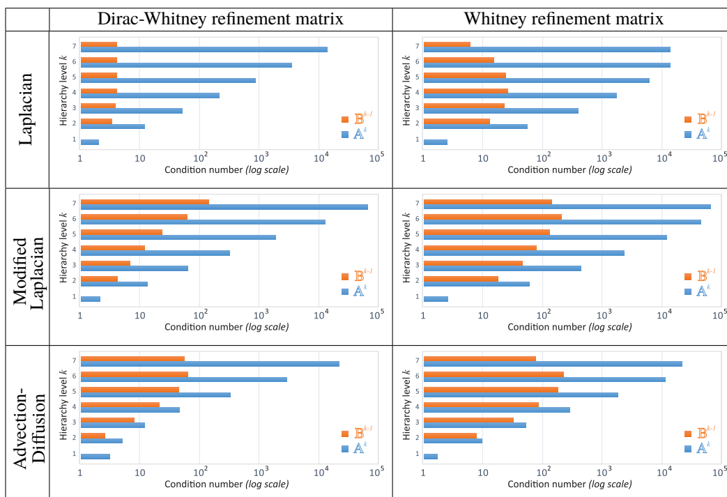
Figure 5.15: Condition Numbers. We compare the condition numbers (in log scale) of stiffness matrices \mathbb{A}^k of 1-form basis functions (in blue) and their associated wavelets \mathbb{B}^k (in orange) for our operator-adapted multiresolution decomposition with q = 7 resolution levels (finest grid is 128 \times 128 cells) for three operators: 1-form Laplacian (top row), modified 1-form Laplacian (middle row, see Eq. (5.28)), and advection-diffusion (right row). The Dirac-Whitney refinement rule (left column) tends to produce slightly better condition numbers for matrices \mathbb{B}^k compared to the original Whitney rule (right column) as expected, but in both cases they remain bounded and often peak on intermediate resolution levels. In particular, condition numbers of the wavelet stiffness matrices \mathbb{B}^k are up to 3 orders of magnitude smaller than those of \mathbb{A}^k for large k (i.e., on finer scales).
