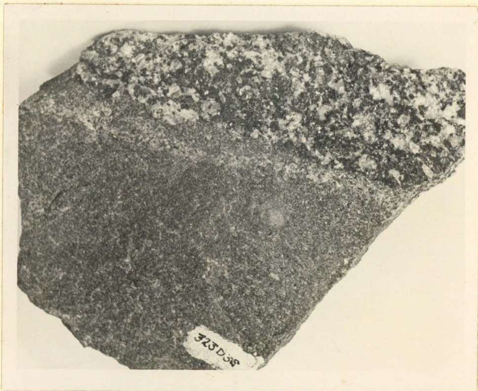
Figure 38. Sacatar quartz-diorite (coarse), with fine-grained inclusion. Near Kennedy meadows. Two-thirds natural size.
