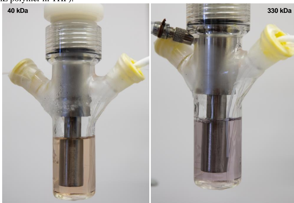
Figure 4.8. Photographs of polymer solutions (2 mg/mL in THF) subjected to ultrasound-induced mechanochemical activation. ( left ) BNP-PMA 40 after 30 min of sonication, and ( right ) BNP-PMA 330 after 9 min of sonication. Immediately after cessation of sonication, the reaction vessel was removed from the cooling bath, sprayed with isopropanol to prevent water condensation, the vessel was illuminated with a fluorescent lamp and immediately photographed. Images were acquired in RAW format to preserve color information.
