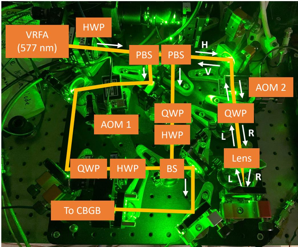
Figure 5.15: The annotated acousto-optic modulator (AOM) setup used to generate two-photon light. White arrows label optical path directions for the double-pass setup. Parts are labeled as follows: VRFA, visible Raman fiber amplifier; HWP, half waveplate; QWP, quarter waveplate; PBS polarizing beam-splitter; BS, 50/50 beam-splitter; H/V, horizontal/vertical polarization; L/R, left/right handed circular polarization. See main text for details. We thank Yi Zeng for setting up the breadboard.
