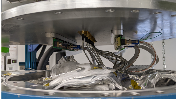
Figure 4.7: Modified 300K vacuum base plate in short K0 included a new RF front-plate that accommodates 8 SMA connectors.
