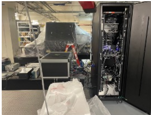
Figure 7.5: Photo of the full setup of LFC. The setup contains one equipment rack on the right, together with two bread boards covered by the black enclosure on the optical table.
