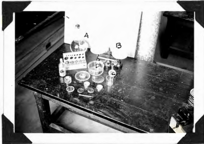
Fig. 9 Shrinkage Limit Apparatus
