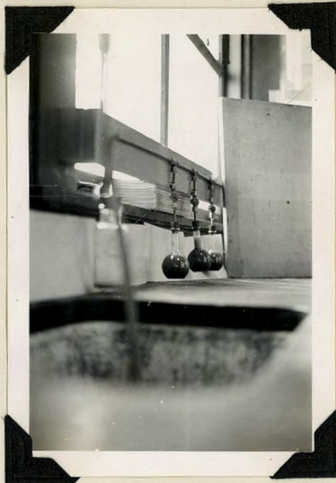
Fig. 10 Specific Gravity Apparatus
