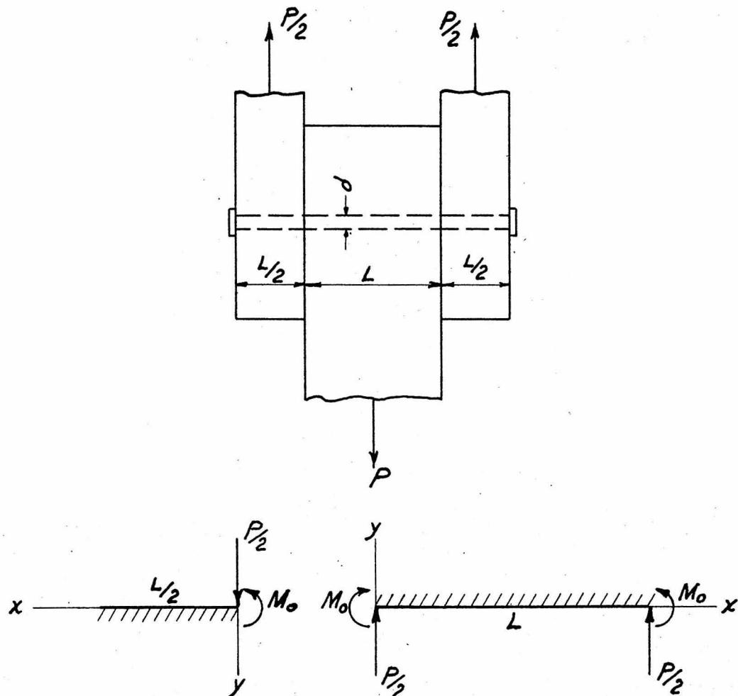
Since the bending of the bolt in the side member must be considered, and since the foundation is discontinuous at the
