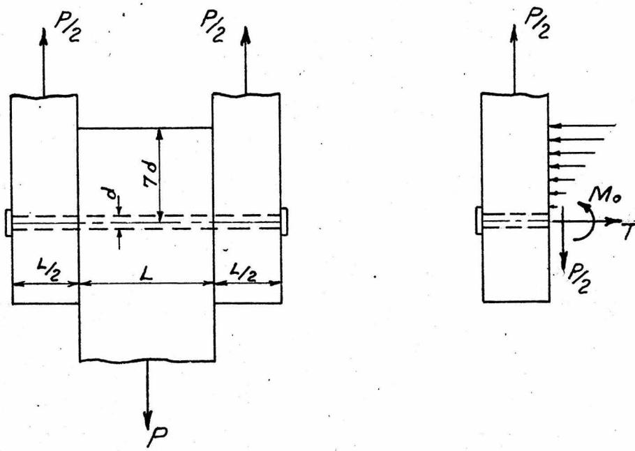
It was stated that under the action of the tension in the bolt, the shear in the bolt, and  $M_0$ , the side member
