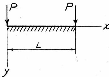
By superposition, using the equation for case 1, the following expression is obtained for the deflection curve of the beam:
