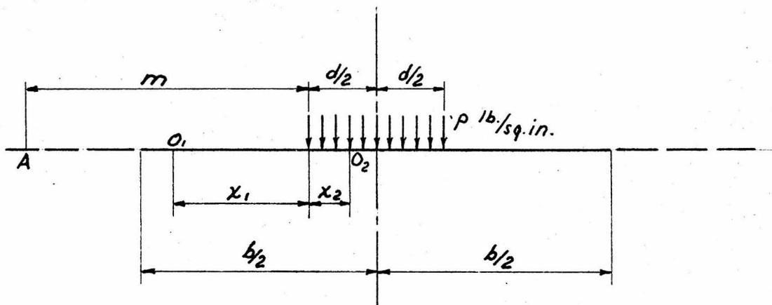
This case may be applied to the bearing of the bolt in a timber if it be considered that the bearing stress is distributed to the wood on a plane through the center of the bolt. Let  $d$  represent the diameter of the bolt and  $b$  the width of the timber through which the bolt is inserted.
