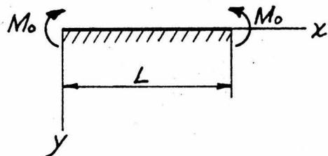
By superposition, using the equation for case 2, there results the following expression for the deflection curve of the beam:
