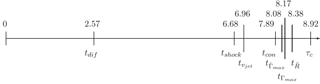
Figure 4.10: Chronology of events in free-field shock-induced collapse ( p_s/p_o = 353 ).
