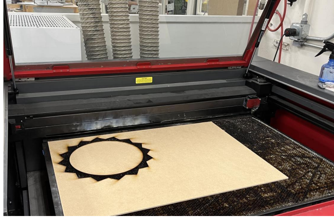
Figure 6.9: The stretching hoop was made from a laser cut wooden board.
