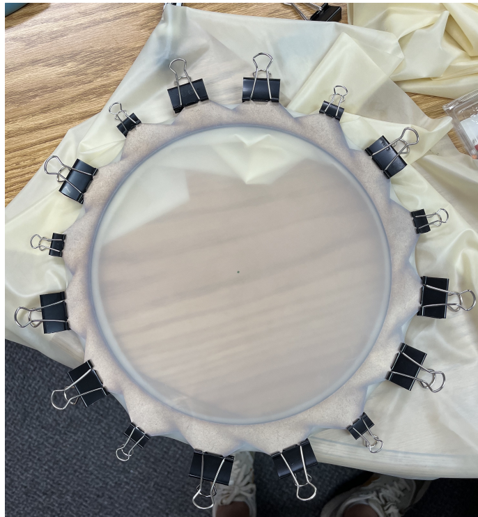
Figure 6.10: Points were measured and marked on the membrane, then stretched along the hoop corners based on the marked points to obtain a corresponding prestretch factor.
