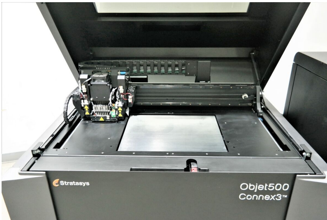
Figure 6.4: The Stratasy's Object500 Connex 3 Polyjet printer used to print the Vero White photopolymer samples.
