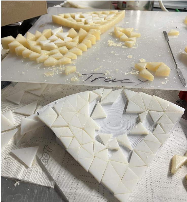
Figure 6.14: The original designs were attempted in the polyjet printer. However the tiles were difficult to clean and retain in their predetermined configurations.
