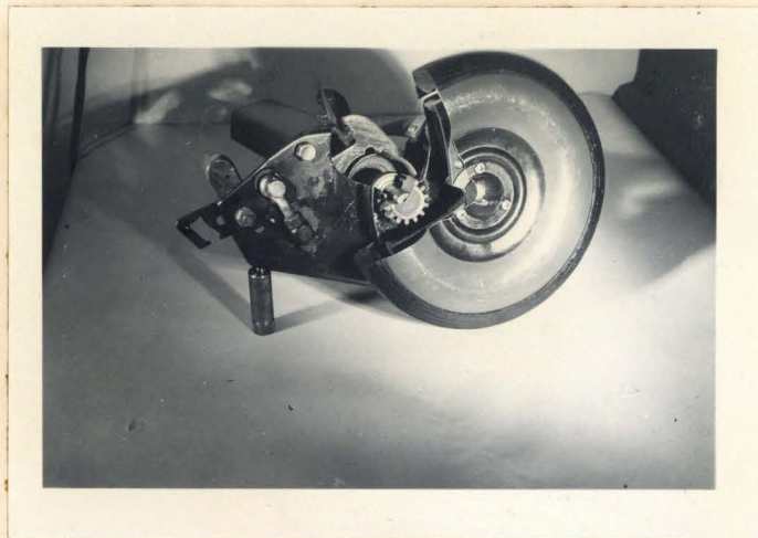
VIEW SHOWING PINION GEAR AND RATCHET TEETH IN PLACE
