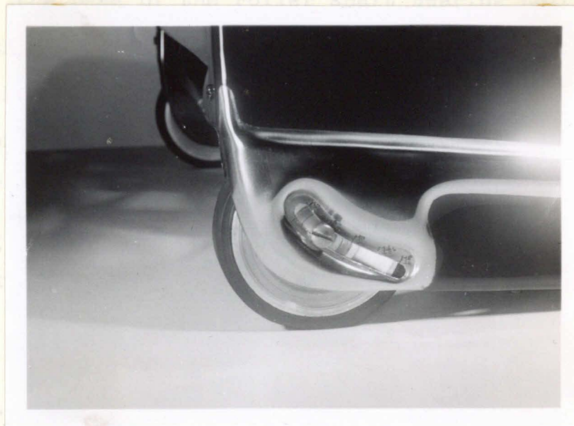
CUTTING HEIGHT ADJUSTMENT AND INDICATIONS
