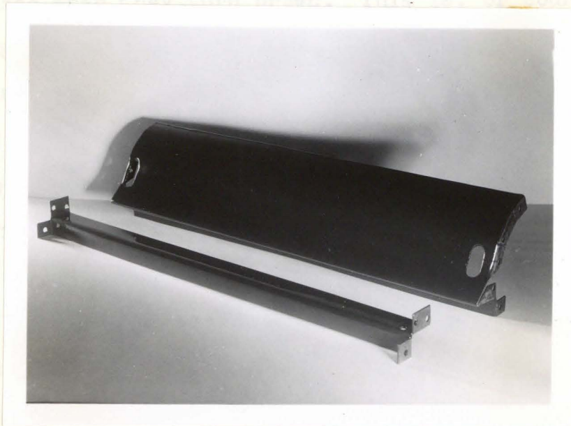
SMALL AND LARGE INTERCHANGABLE REAR CROSS-FRAME MEMBERS
