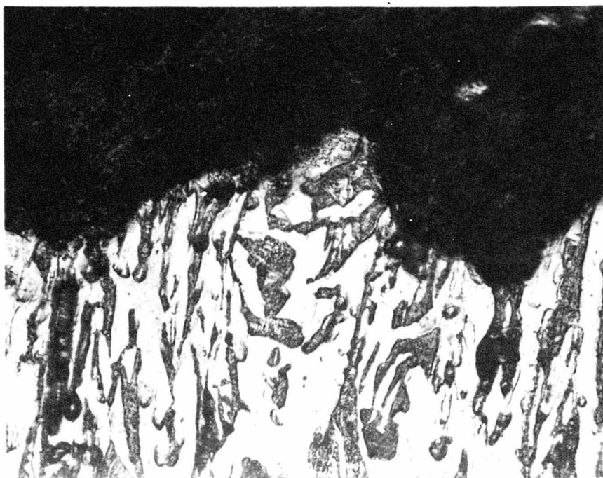
(b) Specimen 92c, ductile fracture at -74^{\circ}\text{F} at impact velocity of 95.2 ft/sec. Nital etch, X300.
