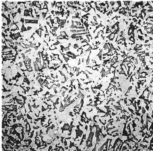
Fig. 3 Photomicrograph of ship plate steel C-10. Nital etch, X100.
