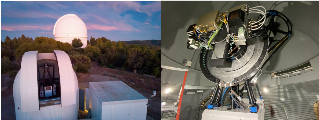
Figure 6.1: The WINTER telescope at Palomar Observatory. Left: A picture of the WINTER dome and 1 m. telescope, with the 200-inch Hale telescope in the background. Right: The WINTER camera mounted on the 1 m. telescope.
