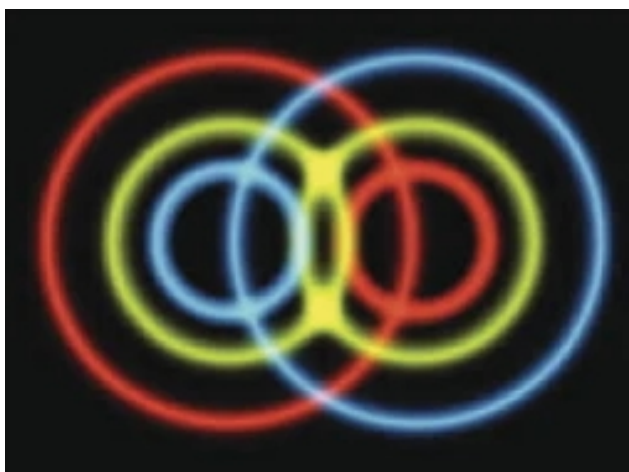
Figure 1.1: Photograph of entangled photons generated from a bulk nonlinear crystal. Three false-color images are superposed. Due to nature of the energy and momentum matching, each frequency is emitted in an emission cone. Reproduced from Ref. [5] with permission from Springer Nature.
