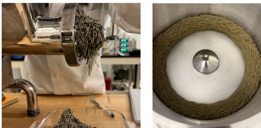
Figure 4.2 displays extrudate exiting the die on the left panel, and sorbent pellets in the middle of spheronization on the right. The extrudate depicted in the left panel is sample A7, which used around a 33% (not yet activated) dry mass of bentonite with a 7.5% dry mass of water added. These “noodles” represent the border of what rods might look like and still be spheronizable. To create fuller noodles more water might be added, or a higher extrusion rate utilized.
