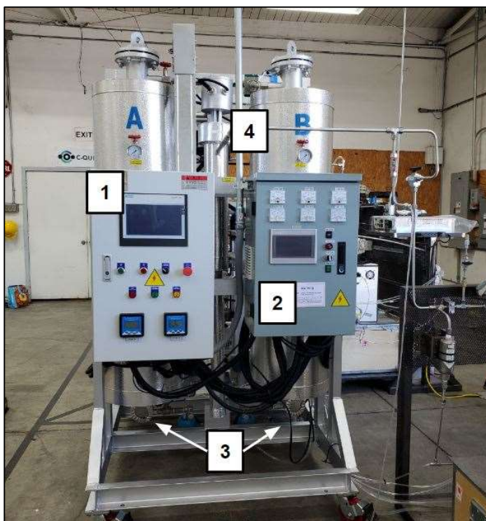
Figure 2.8 displays the front of the two-tower reactor on its mounting skid. The left control panel (1) is used to set and monitor each tower's operating phase (absorption, regeneration, and cooling). The right control panel (2) sets the towers' temperatures. At the bottom of the tower, a set of matching pressure relief membranes are visible (3) that open when tower exceeds pressures of 20 atmospheres. In between towers A and B is an inline heater (4) that can be used to maintain or increase flue gas temperature.
