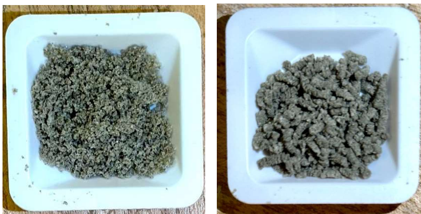
Figure 4.4 displays A6 and A7 after attempted extrusion on the left and right panels respectively. A6 was formulated with an (activated) K_2CO_3 mass load of 75%. Despite its inability to remain in aggregate pieces (it immediately fell apart) the material was quite wet, indicating further water would not improve shape. A7 on the other hand was able to maintain desirable shape with a K_2CO_3 mass load of 60%.
