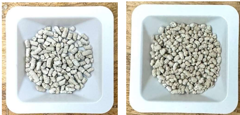
Figure 4.3 shows A1 and A4 after ES on the left and right panels, respectively. Note how A1 maintained a rod-like shape after spheronization due to material stiffness. Extrudate rods or “noodles” also did not break into consistent sizes, generating a variety of granulate lengths. While A4 did not generate perfect spheres after ES, they were more uniform in size and more spherical in shape.
