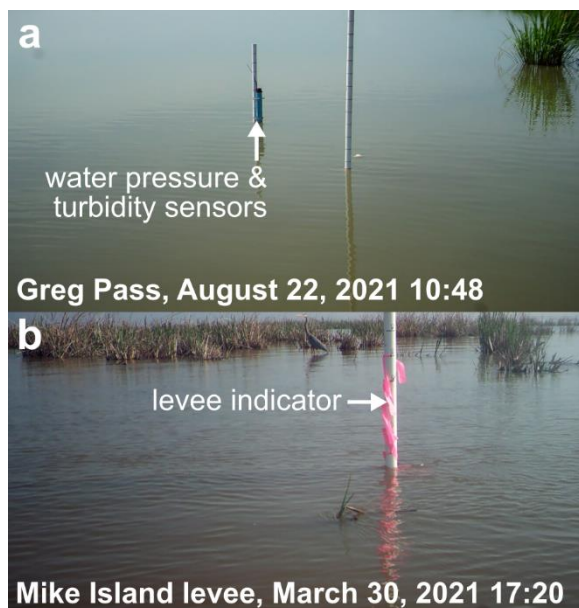
Figure 4. Example photos of in situ sensors. (a) Water pressure and turbidity sensors at the Greg Pass site (Fig. 2e). (b) Levee indicator at the Mike Island levee near the Greg Pass site (Fig. 2e).
