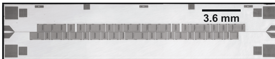
Figure 4.5: Stitched microscope photograph of the 44-pixel chip layout. The single CPW feedline runs in a straight line between the bondpads on the left and right edges of the array.
