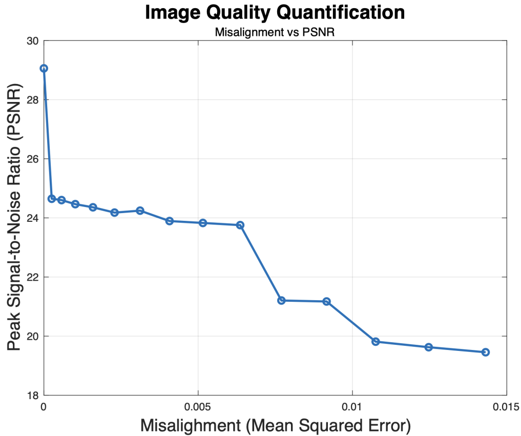
Figure 3.1: Quantification of the effect of misalignment. The PSNR of the image is plotted against the LED misalignment, measured by the mean squared error in k space. There is a noticeably sharp initial decline in image quality for a slight misalignment. For a total shift in illumination accuracy of 0.015 (in k space), which corresponds to a < 0.2 cm shift of the LED, the image quality degrades by up to 10 dB.
