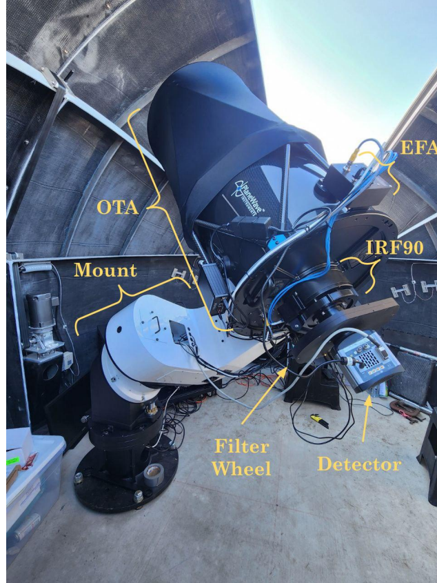
Figure 4.2: Flarescope as it currently exists at Palomar observatory. Several pieces of hardware that I describe in Section 4.2 are labeled here.
