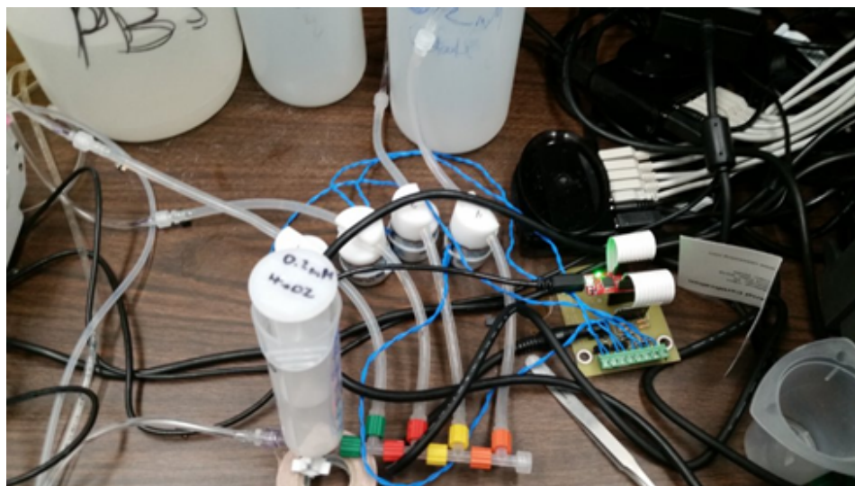
Figure 3.6: Solenoid pinch valves, controller, and fluid source containers
