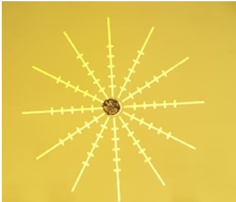
Figure 3.2: 250 \mu\text{m} mechanical mark aligned with lithographically defined feature.
