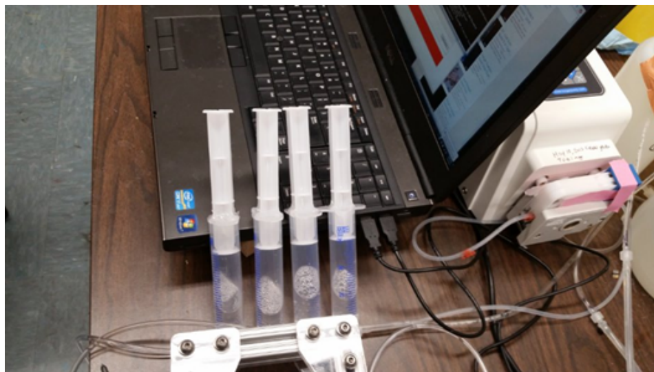
Figure 3.5: Inline flow rate noise dampener comprising of four syringes with plungers fixed in place with adhesive.
