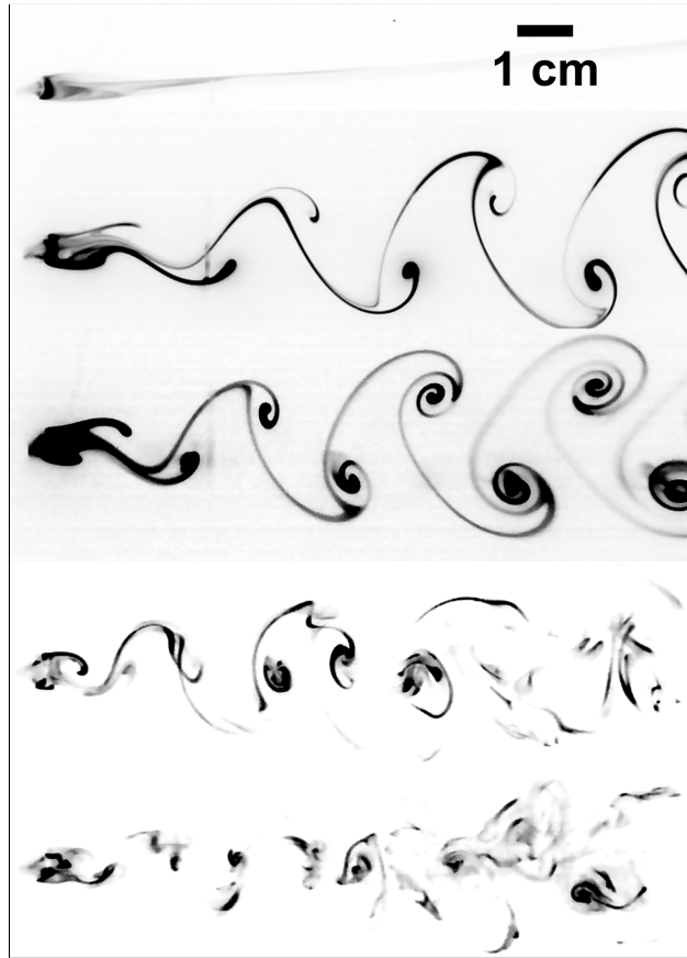
Figure 2.7 Dye visualization of the wake behind a 5.9 mm circular cylinder at Reynolds numbers of 40, 58, 80, 250, and 480 (top to bottom)
