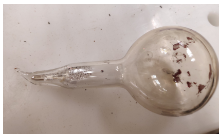
(a) The SEOP cell. Rubidium metal can be seen in the tip.
