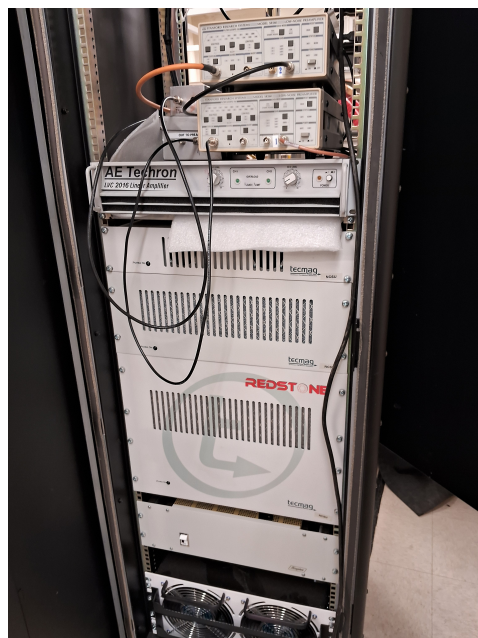
Figure 6.10: Electronics cabinet, including the Redstone NMR system used to perform data acquisition and arbitrary waveform generation. The LVC2016 amplifier and SR560 pre-amplifier are at the top of the cabinet.
