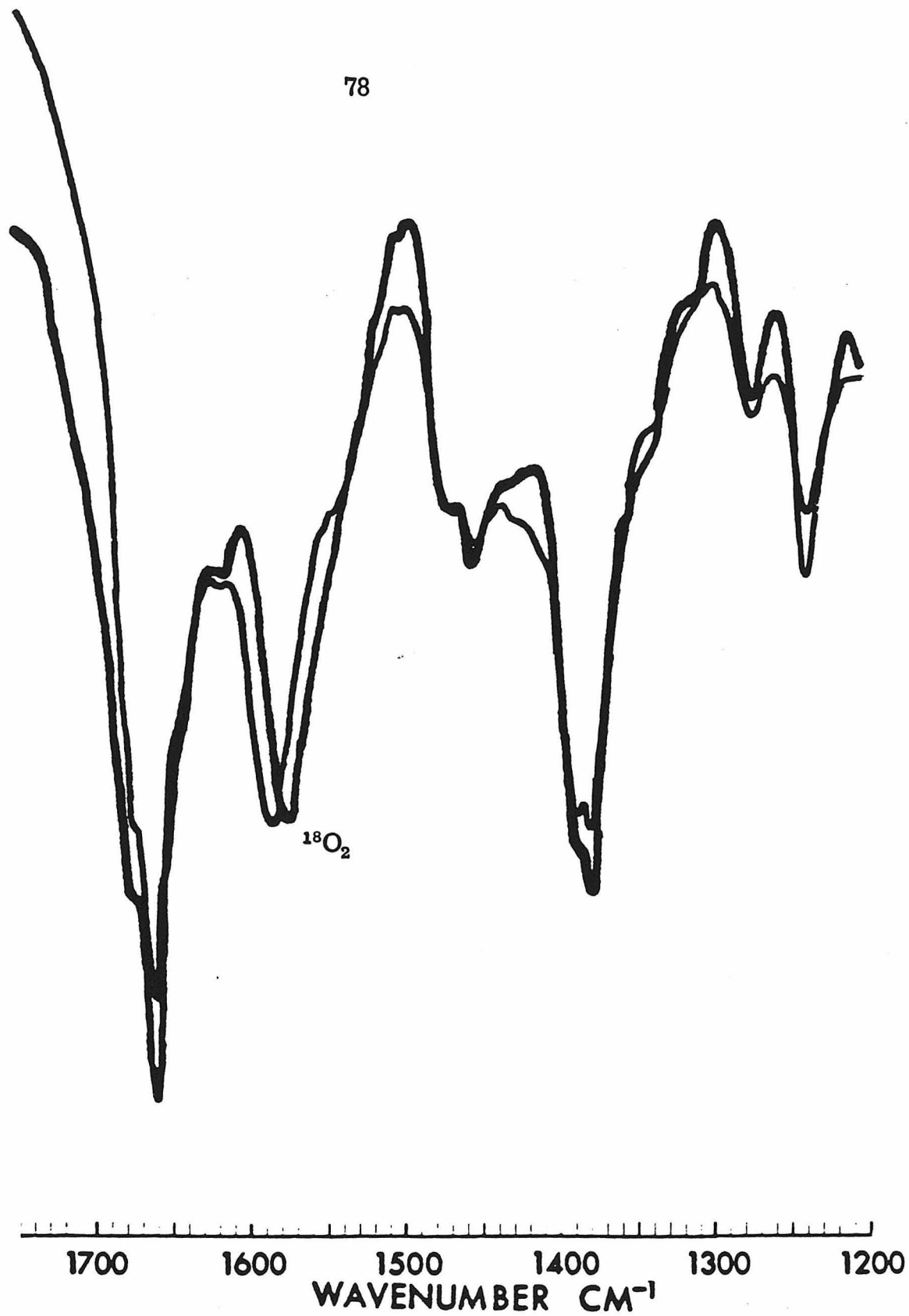
Fig. III-16. Superimposed infrared spectra of the 16 O 2 and 18 O 2 product with Cu(I)Me 8 -tetraene(ClO 4 ).
