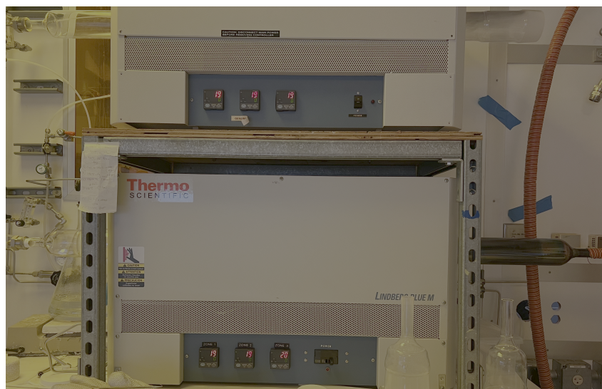
Figure A.7: Tube furnaces used for diffusion doping. The gas lines going to the top furnace currently have a filter attached, while the bottom furnace does not.
