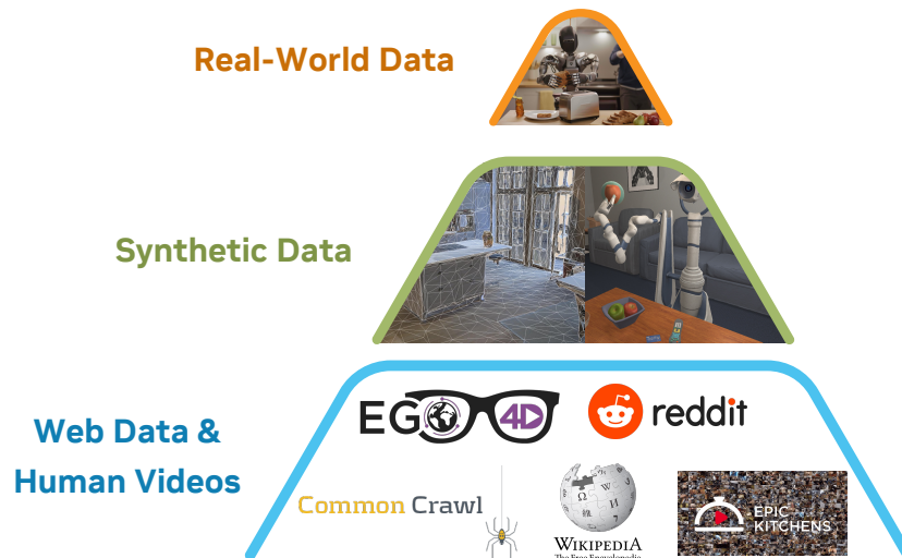
Figure 7.1: Data pyramid for robot foundation model training. GR00T N1’s heterogeneous training corpora can be represented as a pyramid: data quantity decreases, and embodiment-specificity increases, moving from the bottom to the top.
