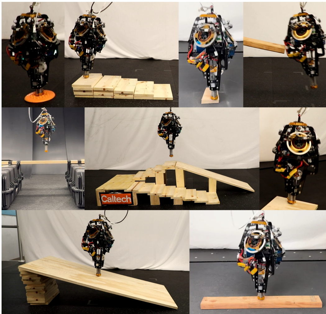
Figure 8.4: A snapshot of the experiments conducted with ARCHER, including set point tracking, disturbance rejection, and hopping over rough terrain.
