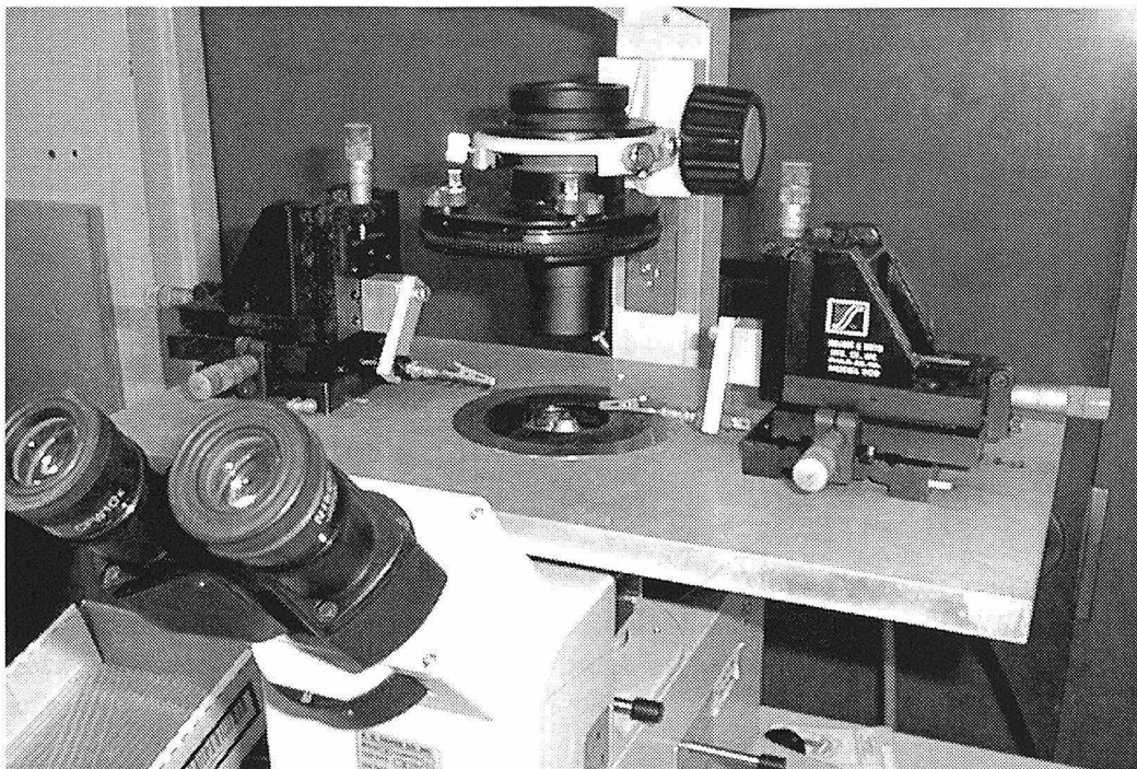
Figure 4: photograph of the microscope with XYZ stages
