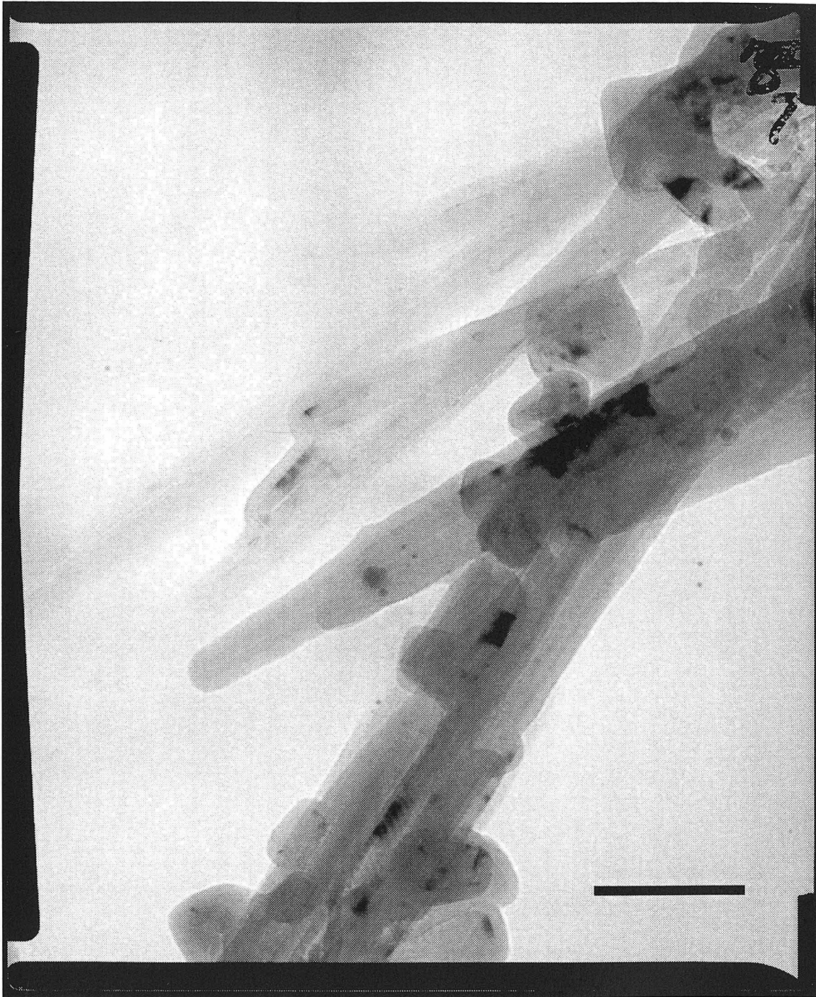
Figure 7b: Control sample prepared identically to 7a. 280,000 X. Again, gold balls are very rare. The scale bar is 100 nm.
