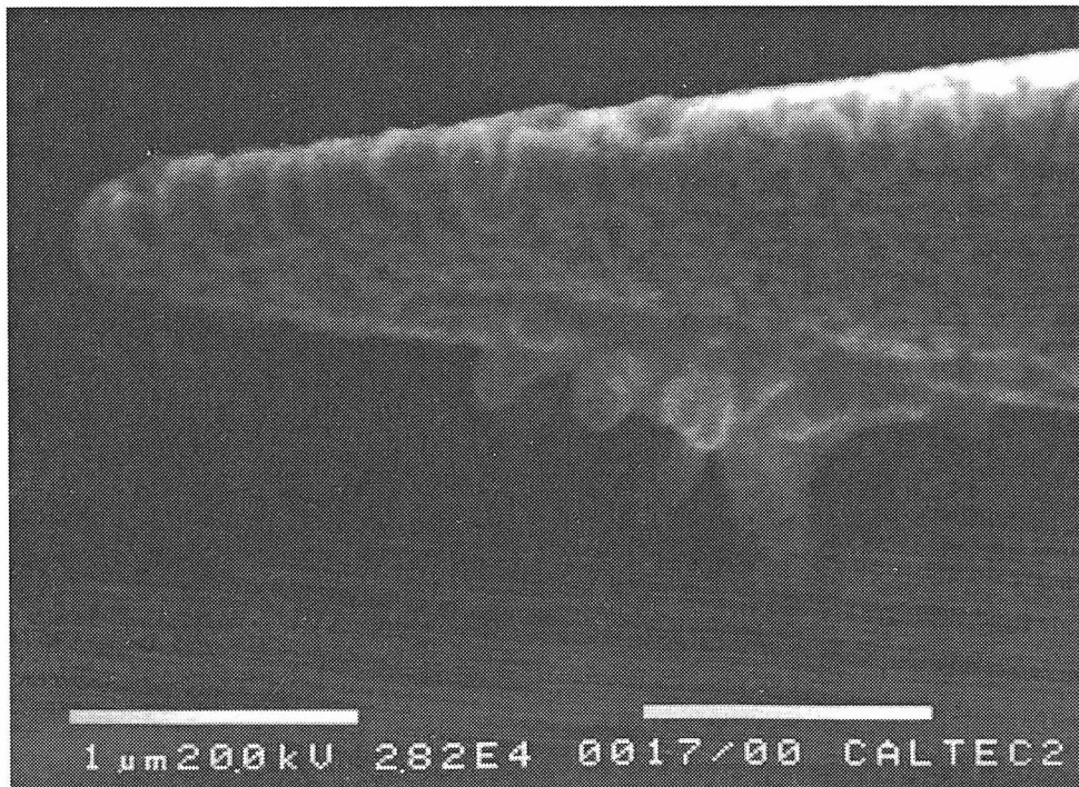
Figure 6: Zoom onto the apex of the tip shown in Figure 5. Scale bar = 1 \mu\text{m} . The corrugations and the structure on the underside of the tip are believed to be due to the thin layer of gold applied for SEM imaging.
