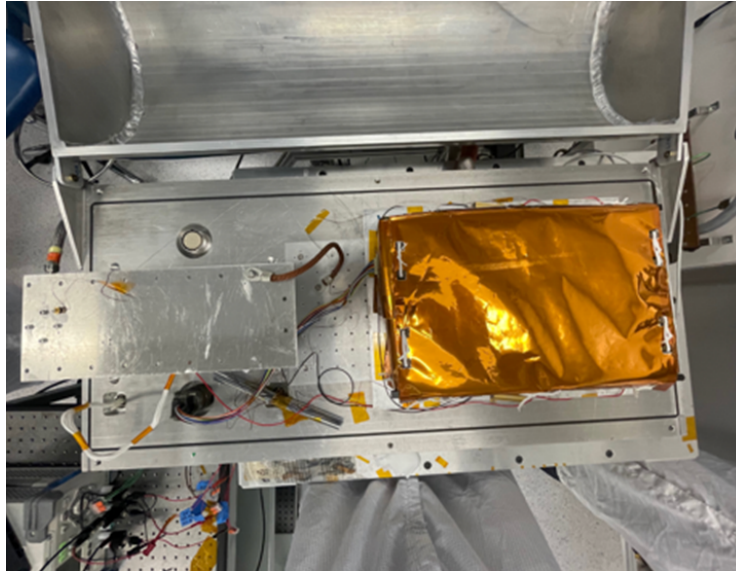
Figure 4.14: MAPLE EM mounted for TVAC testing at JPL post-mission
