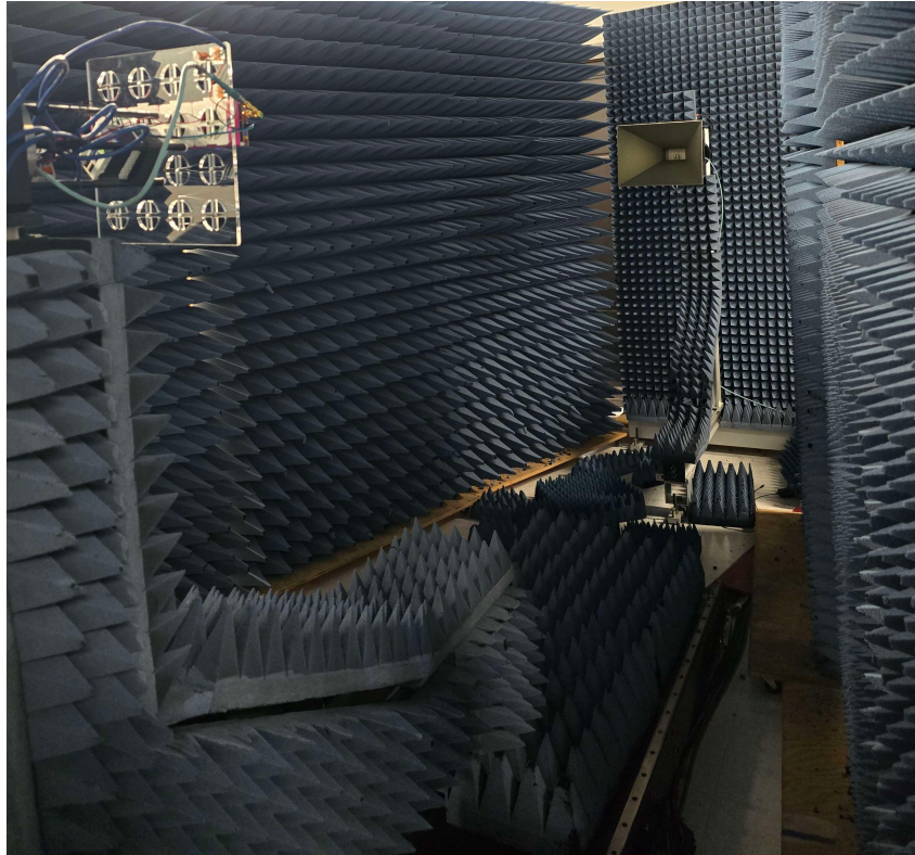
Figure 3.2: An example of a far-field range measurement in an anechoic chamber
