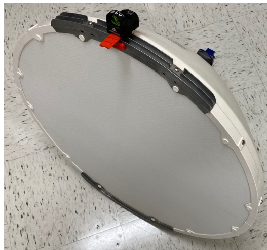
Figure 2.21: Dish antenna with optical sight fixed at the top.
