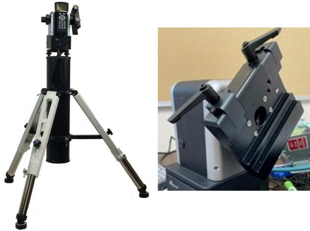
Figure 2.17: Dish antenna equatorial mount.
