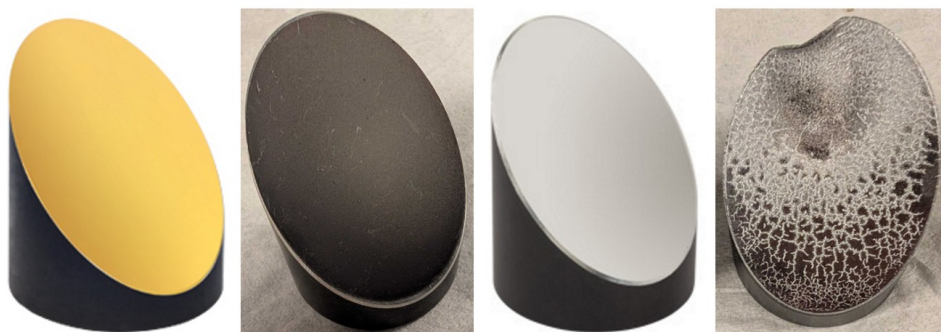
Figure 4.7: Mirror failures caused by thermal runaway. From left to right: New gold-plated concave aluminum mirror [257], damaged gold-plated mirror, new protected aluminum mirror [257], damaged protected aluminum mirror.
