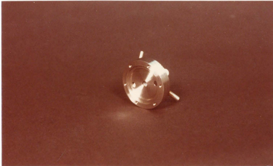
d) PROFILE OF D-SIDE -- Female sealing surface; 2mm deep gas chamber.
