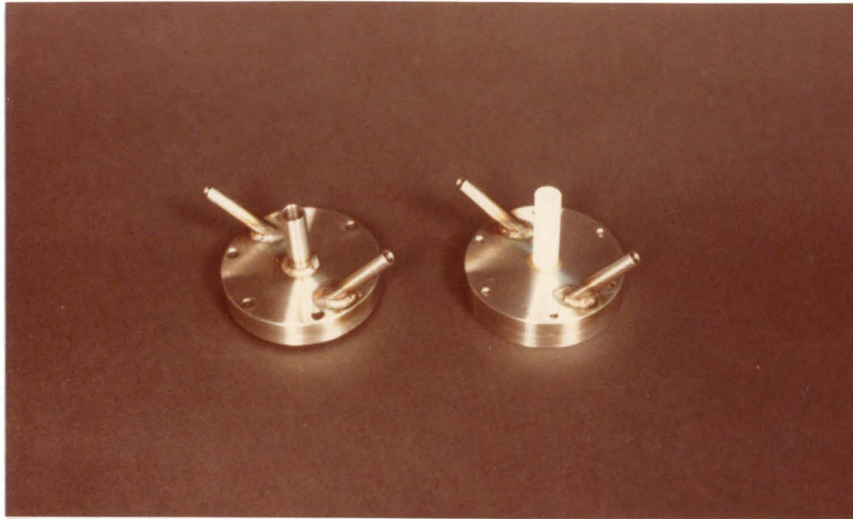
a) TOP VIEW -- Inlet ports placed to produce swirl; exhaust ports centered; six holes for screws.
