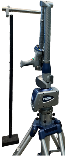
Figure 2.3: Longeron in Set 2 suspended vertically for scanning.
