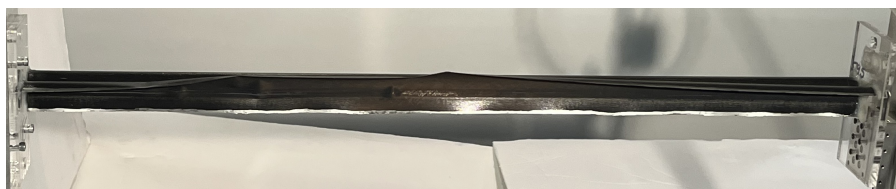
(b) Back flange in compression, Sample 1
