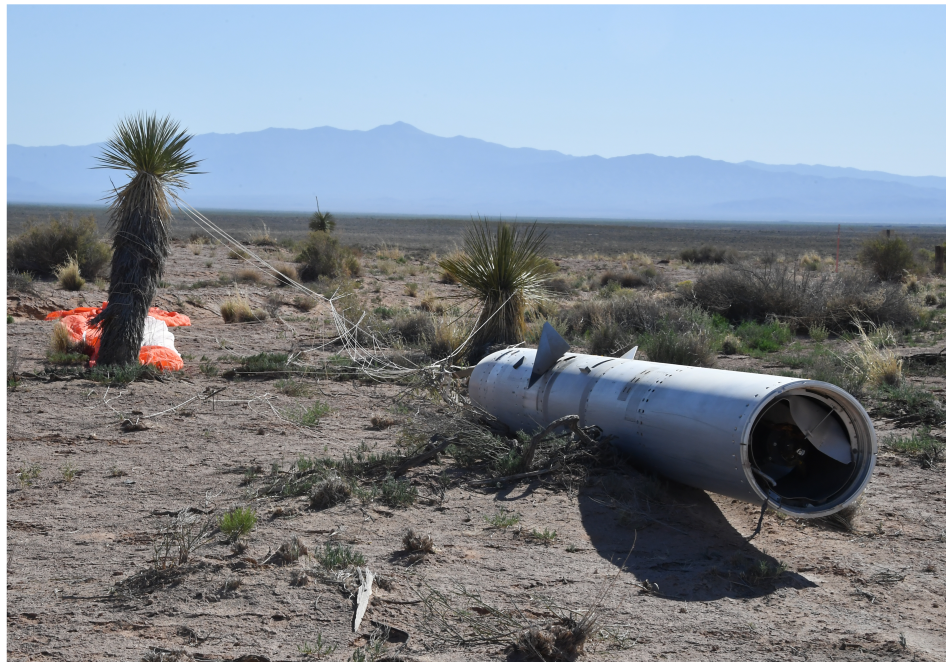
Figure 3.11: CIBER-2 as recovered after the 3rd flight on May 6, 2024, far from its original touchdown site. Note damage to the pop-up baffle. The detectors and warm electronics suite were unharmed, and all flight data was successfully recovered later that day. Photos: NSROC
