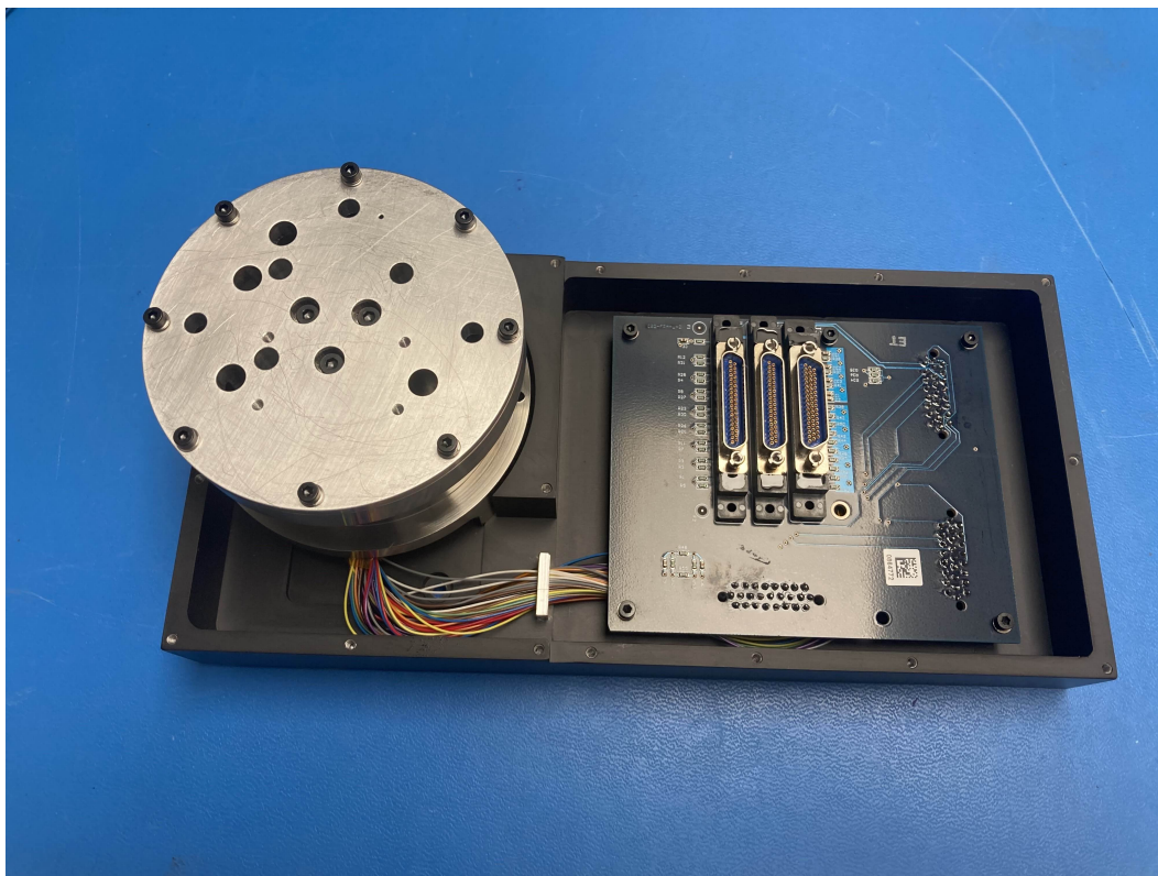
Figure 3.22: The final fully assembled long-wavelength focal plane array, lacking only the anodized aluminum cover that normally conceals the focal plane readout board. All openings in the aluminum base plate (top left) as well as seams on the anodized housing were covered in mylar tape prior to integration into the overall instrument to prevent light leaks. The custom focal plane readout board (right) breaks the H2RG signal output into three standard connectors that can be accessed without opening the FPA, routing to the main CIBER-2 warm electronics suite.
