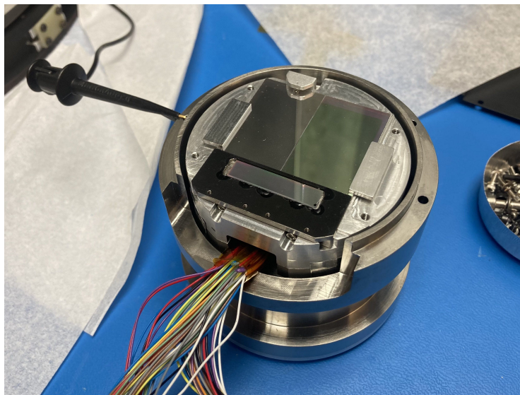
Figure 3.20: The fully assembled FPA stack after integration into the titanium housing, with both filters covering the H2RG surface visible. Dust on the filters, an inevitability even in a cleanroom environment, was removed with a squeeze blower prior to integration into the overall instrument. Note the gap between the aluminum top cap and the titanium housing, providing thermal stability for the H2RG by forcing all heat transfer to occur only through the housing, aluminum base plate (not visible), and molybdenum mount (not visible).
