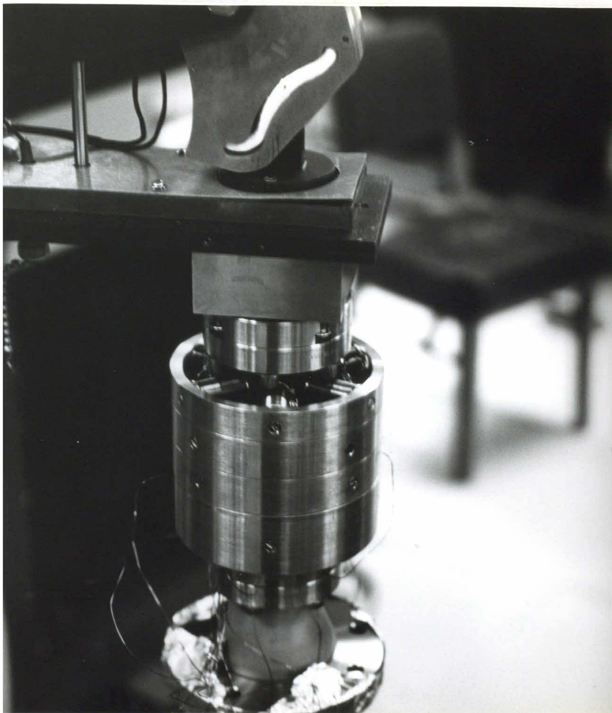
Figure 5.3: Photograph of the magnetic lens system employed in the parallel REELS assembly. The coils of the sextupole lens are visible.
