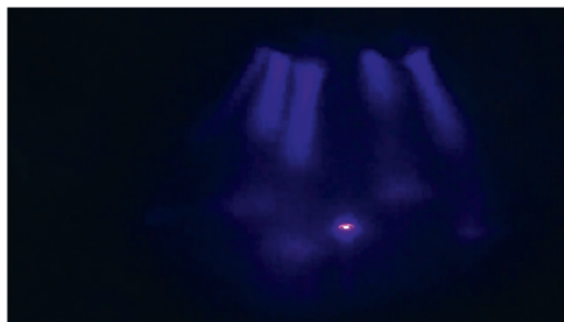
Figure B.9: Movie S2 Effect of high electric potential on the plasma stability and viability. The movie was taken from the impinging side and shows that the application of a 50\text{ kV} potential between the wafer and the nozzle, either positive or negative, leaves the plasma structure unaffected. The luminescence was generated in a mixed atmosphere of air and helium. Secondary streamers are seen that bridge the nozzle to the wafer away from the luminescent structure at the jet impingement site. They are not connected and do not interfere with this latter phenomenon.
