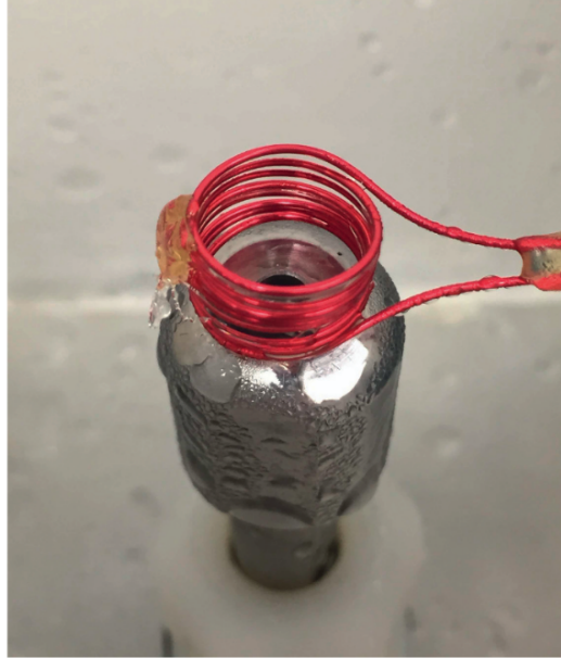
Figure B.2: RF antenna. The customized RF antenna is shown in its setup position relative to the jet nozzle. The antenna axis is collinear with the jet axis.
