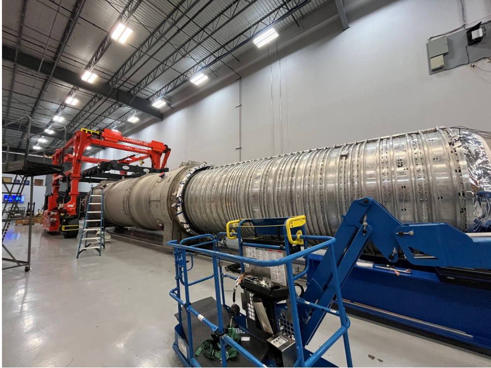
Figure 2.21: The Detector Solenoid cold mass being inserted inside the vacuum vessel at the vendor factory (in October 2025)
