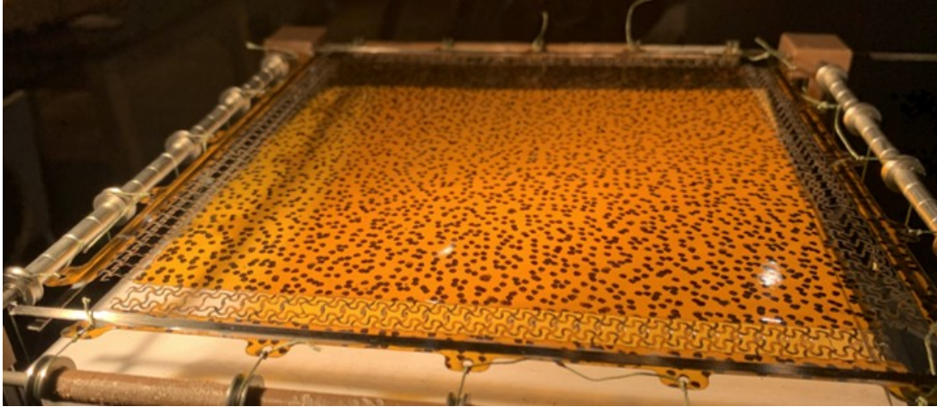
Figure 4.4: A frame made of four battens pretensioned by pulleys. The film surface can be observed to be smooth, and the double s-springs along the edges displaying post-buckling behavior.
