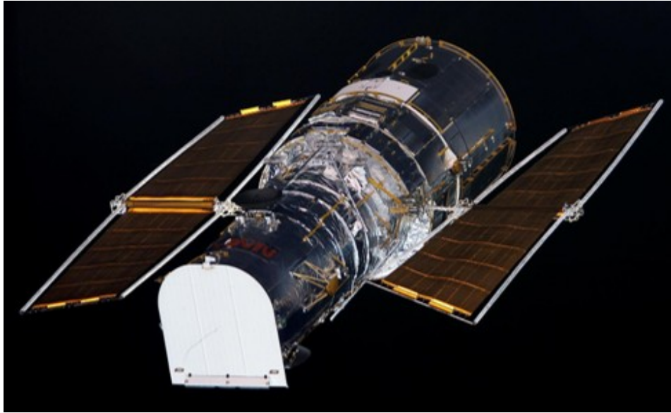
Figure 1.3: The Hubble Space Telescope's second set of solar arrays undergoing torsional buckling due to thermal changes (Copyright ESA).
