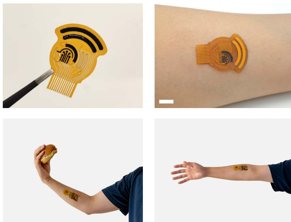
Fig. A-1. Images of the wearable cardiometabolic tracking patch. Photographs showing the fabricated epidermal lipid-profiling patch used for continuous cardiometabolic monitoring. Scale bars, 10 mm (top row), 100 mm (bottom row).
