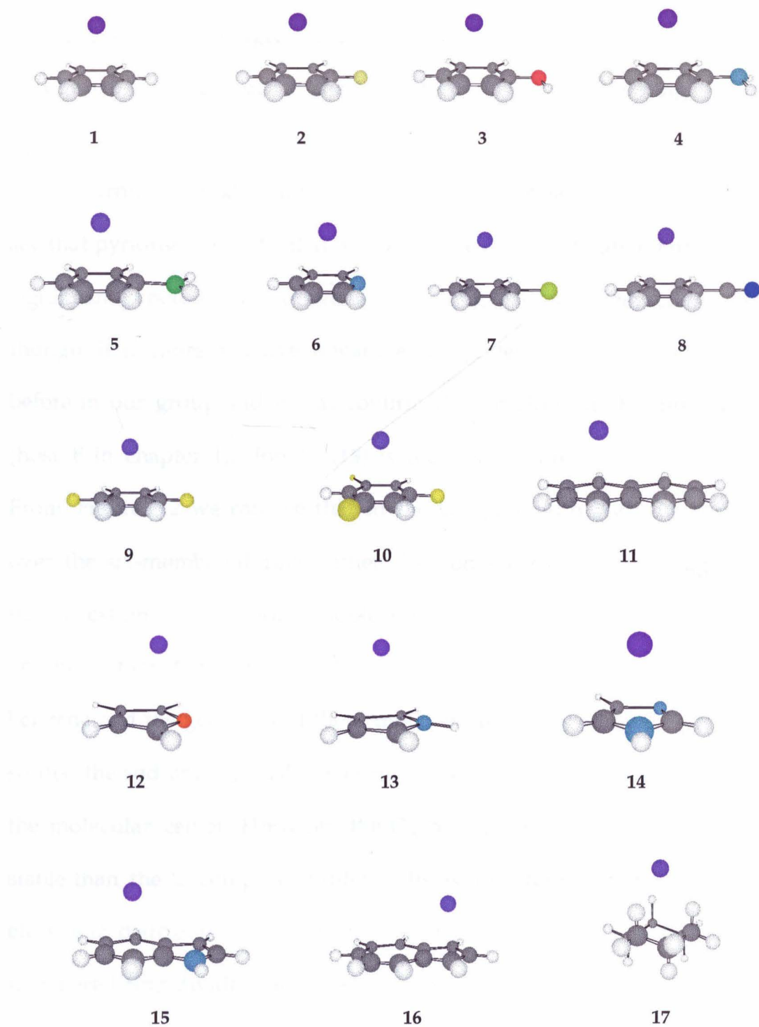
Figure 3.2. Structures of the optimized complexes between aromatics 1-17 and \text{Na}^+ .
