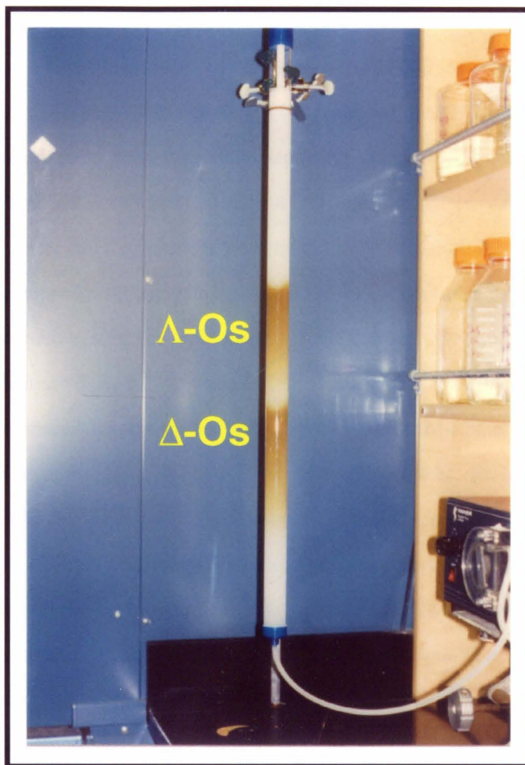
Figure 2.19. Sephadex SP-C25 cation exchange column used to resolve rac - [\text{Os}(\text{phen})_2(\text{dppz})]^{2+} with bis -tartrato diantimonate (aq; 0.15 M) as the chiral eluent. The resolution was complete when the two bands were separated by column support that was essentially free of metal complex. The first band that elutes is the \Delta enantiomer, which is followed by the \Lambda complex. The assignment of absolute configuration was made by comparative CD studies between the bands isolated here and the CD spectra for the pure enantiomers of [\text{Ru}(\text{phen})_2(\text{dppz})]^{2+} .
