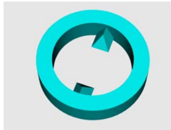
Figure 4-2: Bluff-body stabilized burner flameholder detail, viewed from the upstream side.
