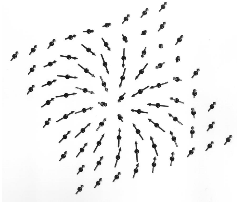
Fig. 7.1. Sketch of a single skyrmion showing the electron spin configuration (arrows) versus position in the 2D plane.
